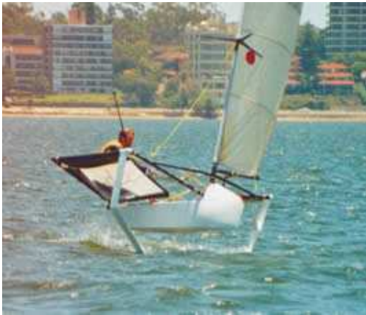
Early hydrofoils mounted from the wings.
