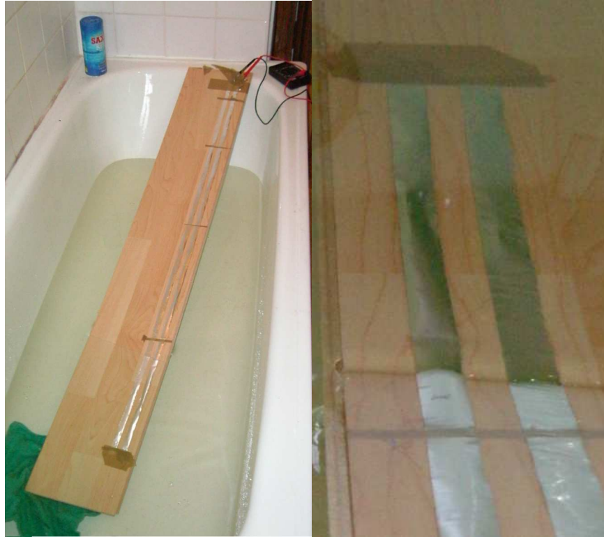
The setup for testing metal strip sensors. The left picture is the strips taped to the MDF board, while the right picture shows a close up of the strips.
