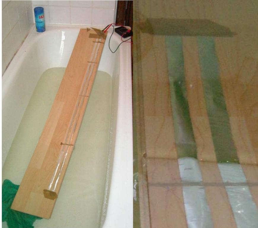
*The setup for testing metal strip sensors.
