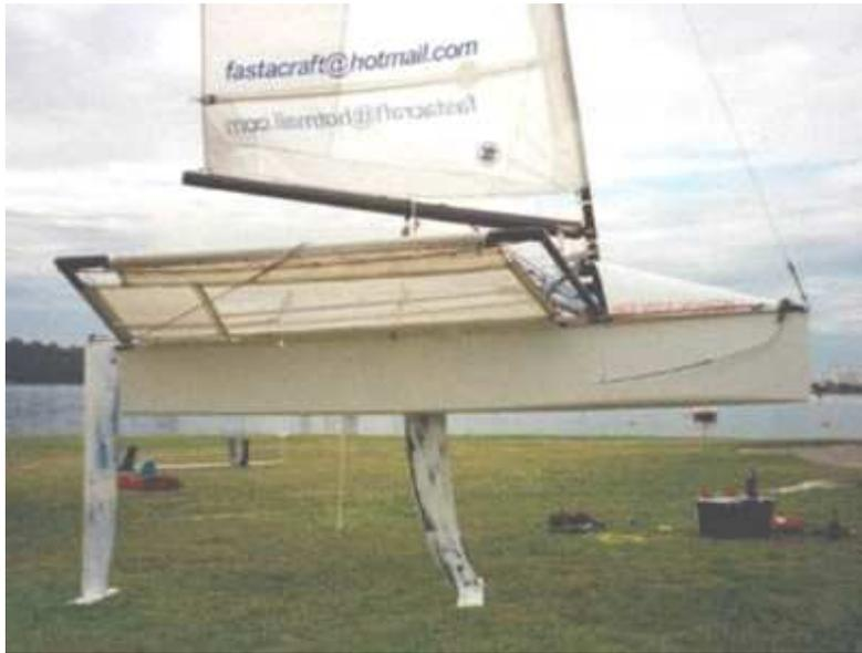
*Prowler design of moth with foils mounted on the dagger board and rudder out the water.*
