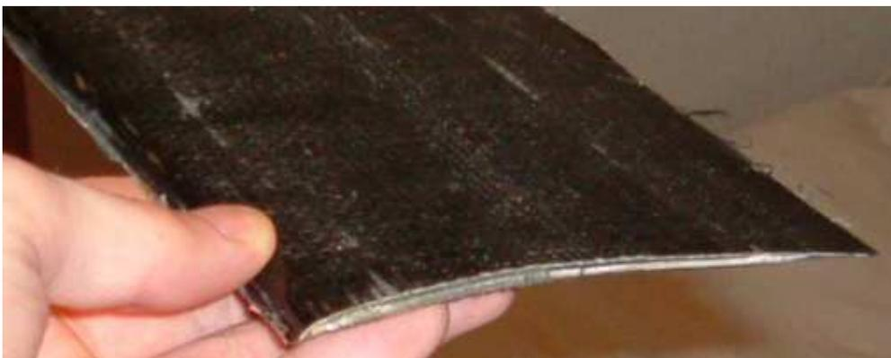
*This is the final section. The different layers can just be made out. Note how the balsa finishes before the trailing edge. This is because the trailing edge is very thin.*
