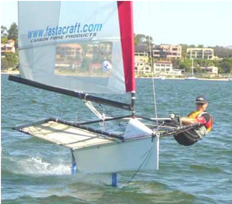
Garth Illett foiling with the hydrofoils attached to the dagger board and rudder only.
