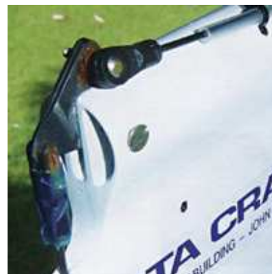
Bow arrangement of Fastacraft moth. Note the use of a power boat throttle cable for the control cable.
